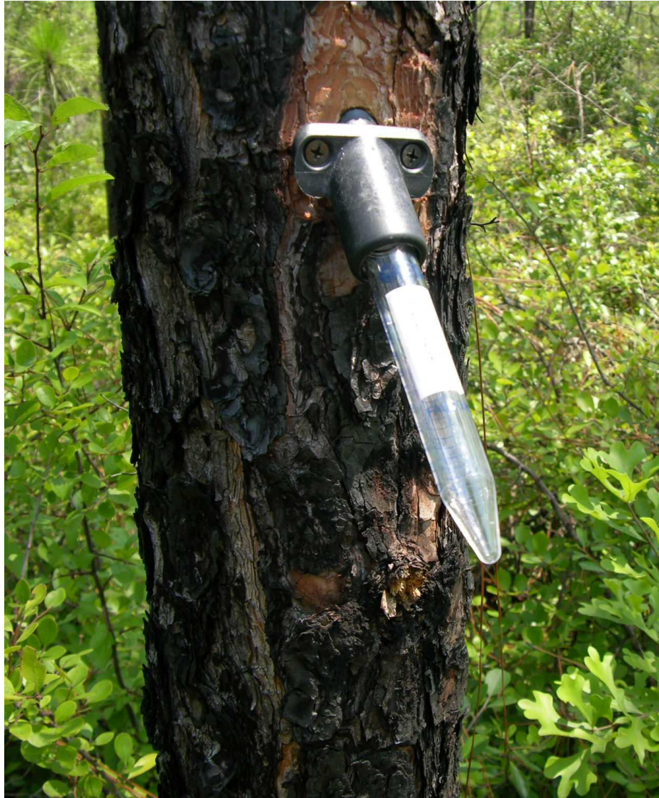
Figure 2.3. Resin collection apparatus, in situ.
